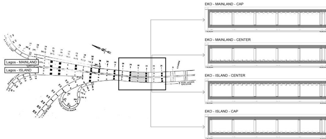
Figure 5: Sensor positions for the 4 applied measurement arrays at the Eko Bridge.
